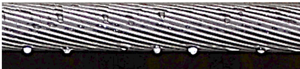
Fig. 3: Conductor surface with prominent water drops (new standard conductor)
