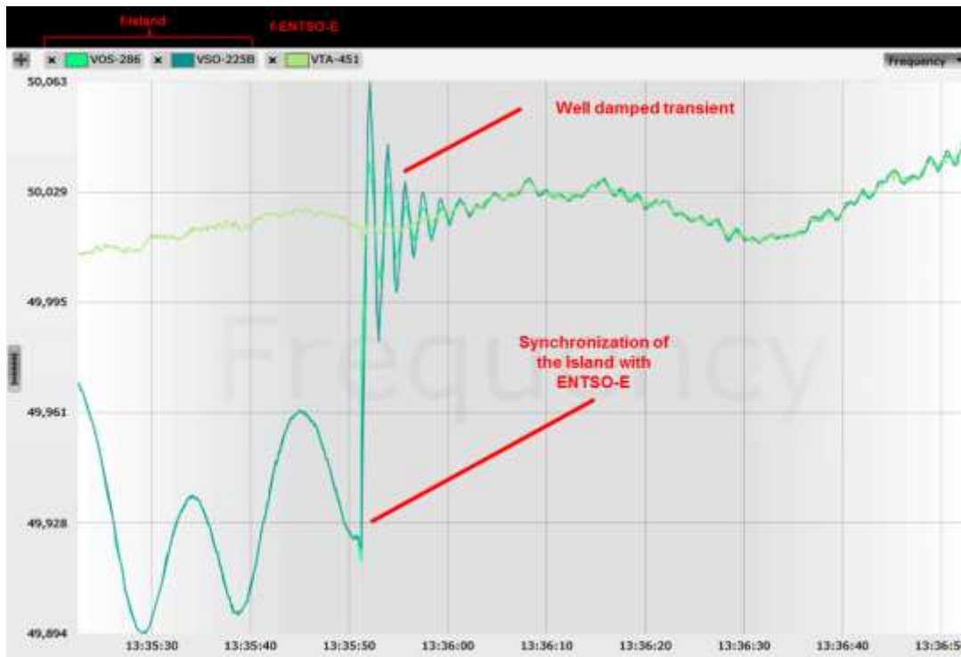
Figure (5) Synchronization of the islanded system with ENTSO-E
