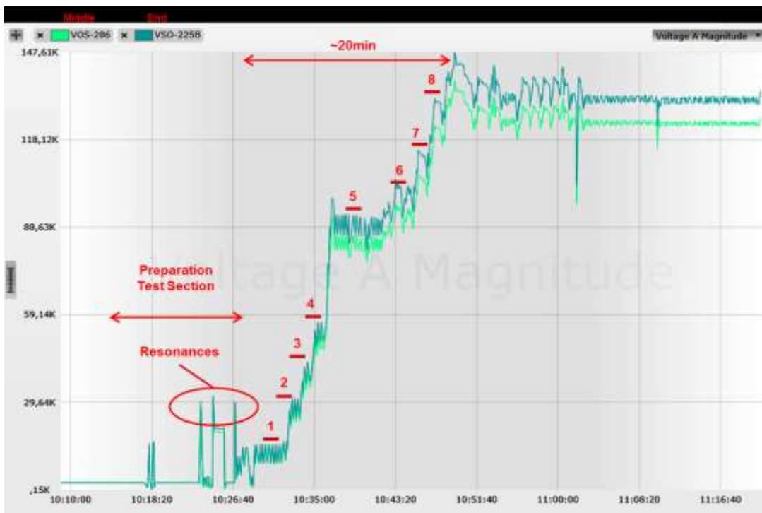
Figure (2): Disconnection of test section from superior grid, voltage ramp, measured at in the middle and at the end of the test section
