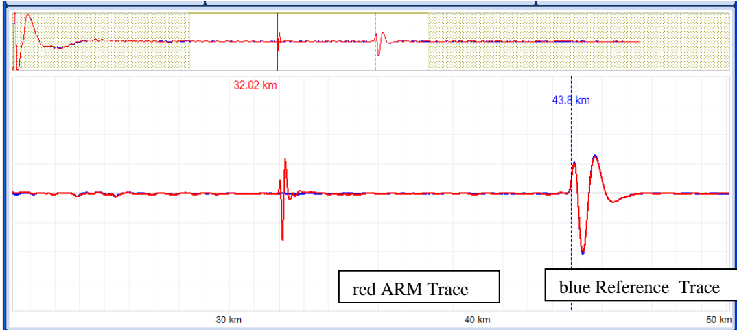
Figure 7: Fault located with ARM at 32 km distance
