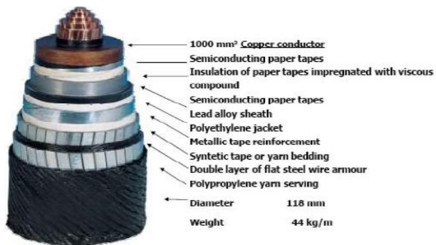
Cable for medium-shallow water Manufacturers Prysmian, Nexans
