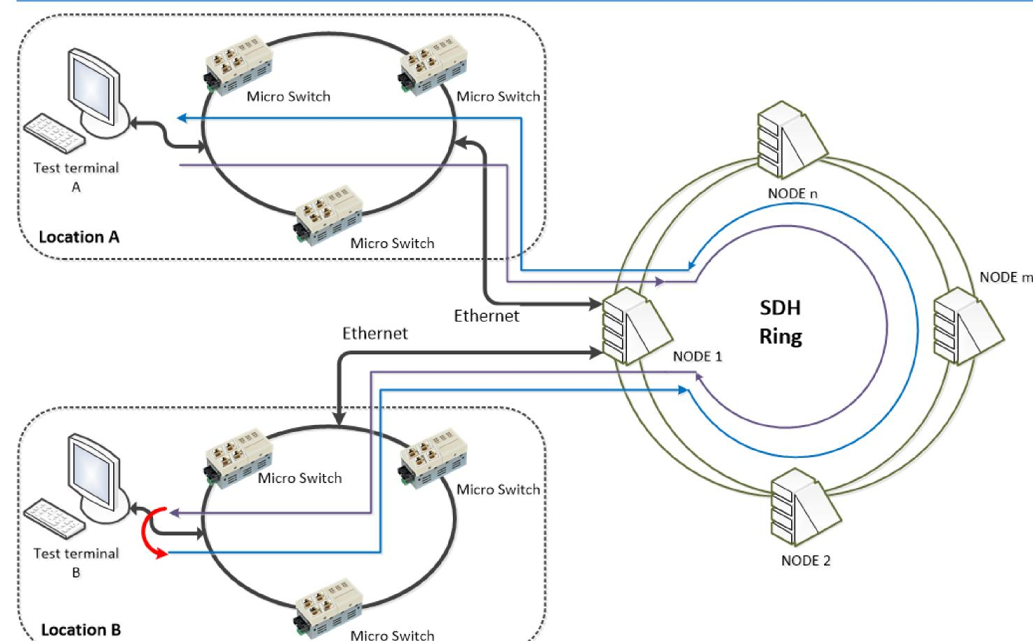
Dedicated (unicast) and GOOSE (multicast) messages were generated by the software using protocols from the second and third layer of the OSI model.
