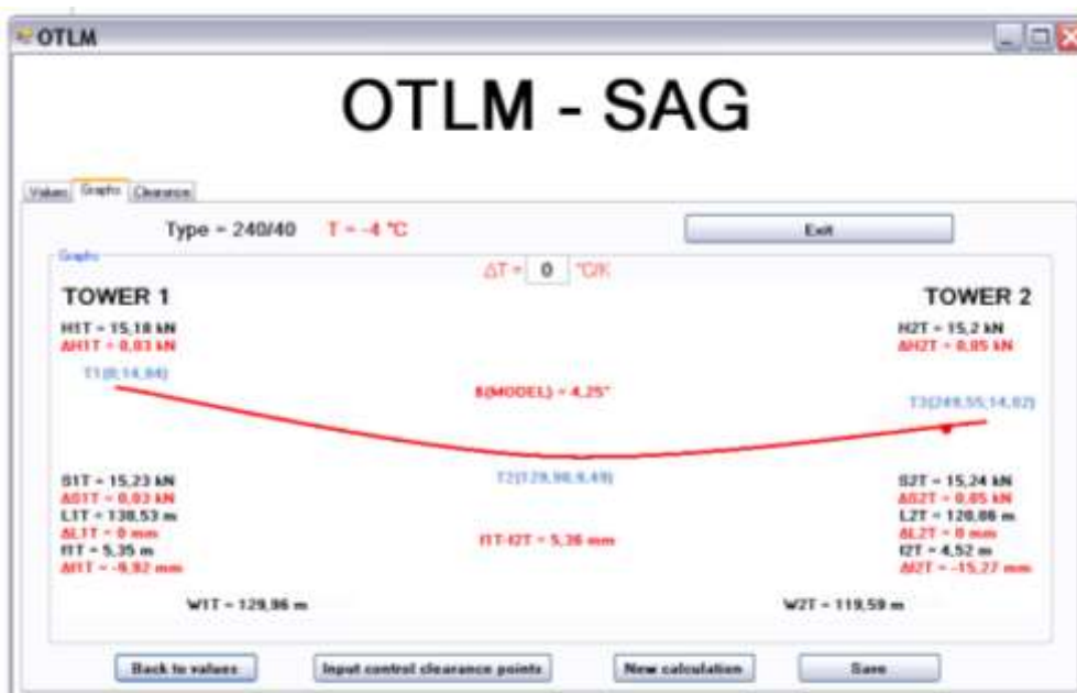
Figure 9: Calculated parameters of the catenary curve and axial tensile forces in the conductor at the temperature of freezing rain without the ice load
