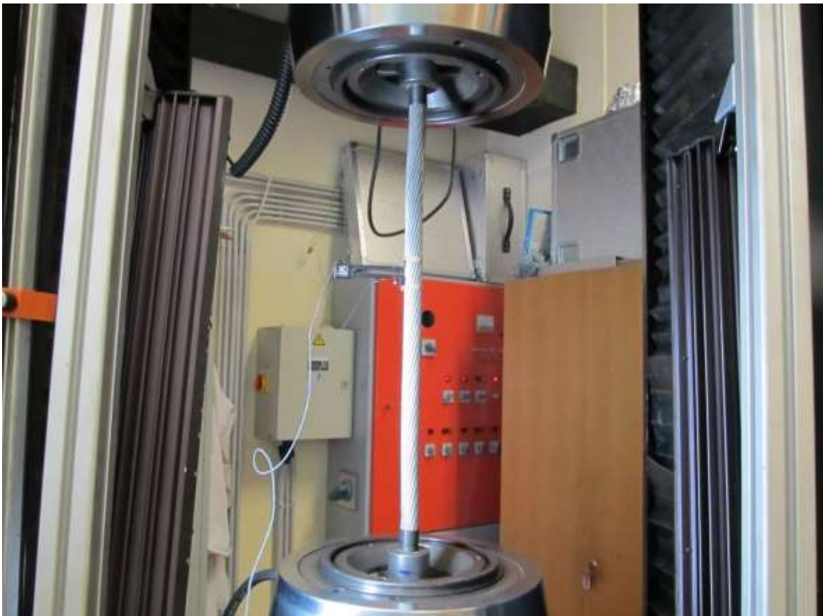
Figure 2: Tensile testing of the conductor in a laboratory
