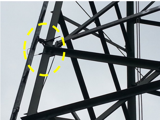
Figure 3: Layout of accelerometers in both directions in relation to the plane of the profile
