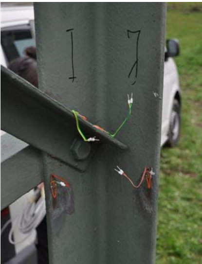
Figure 1: Layout of strain gauges on the south-east tower leg
