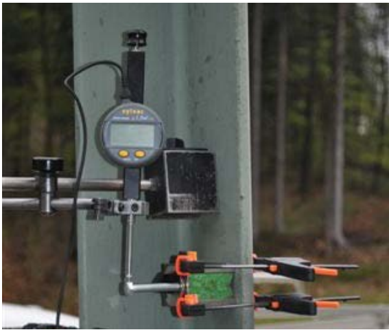
Figure 2: The control penetrometer was placed on the south-eastern leg
