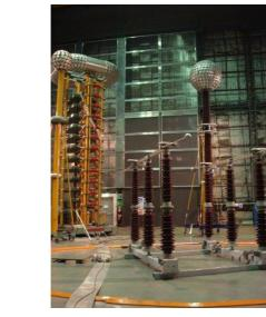
Fig. 2 Two pole disconnectors with double open gap - set up for dielectric test
