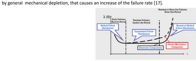
Fig. 9 Comparison bath curve for electronic and electromechanical components [18] [19]
