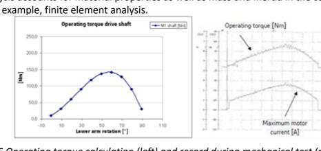
Fig. 6 Operating torque calculation (left) and record during mechanical test (right)
