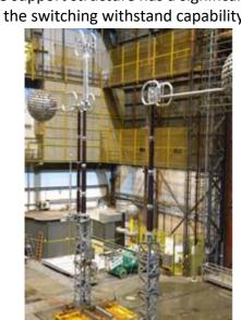
Fig. 1 Single pole disconnector with single open gap - set up for dielectric test
