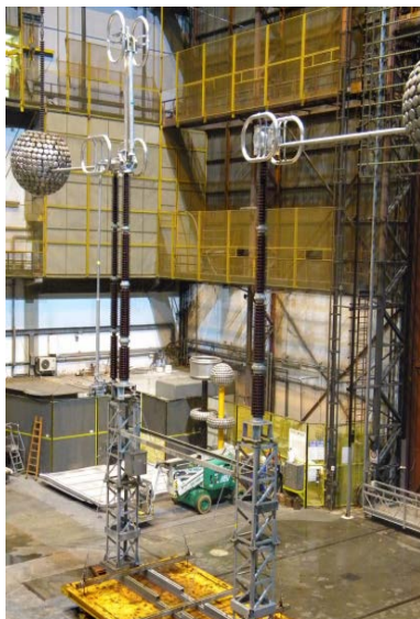
Fig. 1 Single pole disconnector with single open gap - set up for dielectric test
