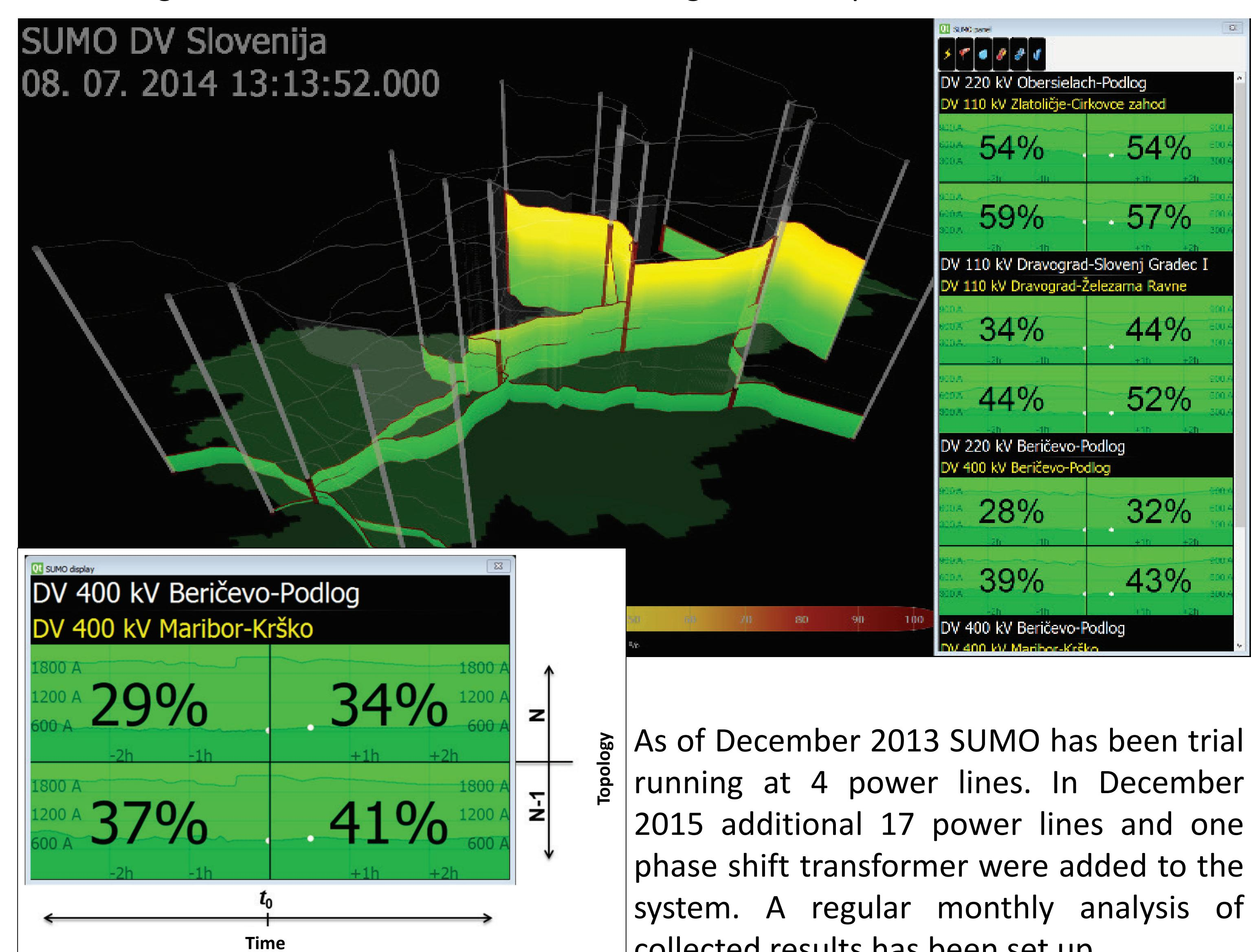
As of December 2013 SUMO has been trial running at 4 power lines. In December 2015 additional 17 power lines and one phase shift transformer were added to the system. A regular monthly analysis of collected results has been set up.
